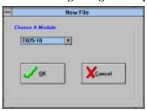
■ Click on the arrow in the square box at the right of the current T800 module. A drop down list box appears with a list of T800 modules which can be programmed.
